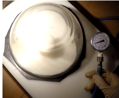
Figure 35: Removing air bubbles from the Epoxy using vacuum.
