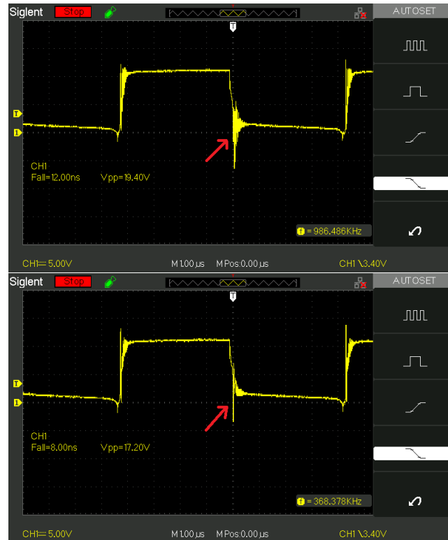
Figure 25: Waveform comparison at Mosfet gates. Up: only diodes. Down: diodes in series with 100\Omega resistors.
